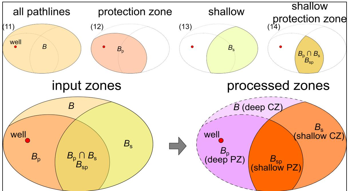
Figure 8: Processing zones from backwards particle tracking results from FEFLOW simulations. Notations used to describe each zone are described in Table 10. In the 'processed zones' subfigure, the four names (in parentheses) and styles are the same as used for maps in the results section.
