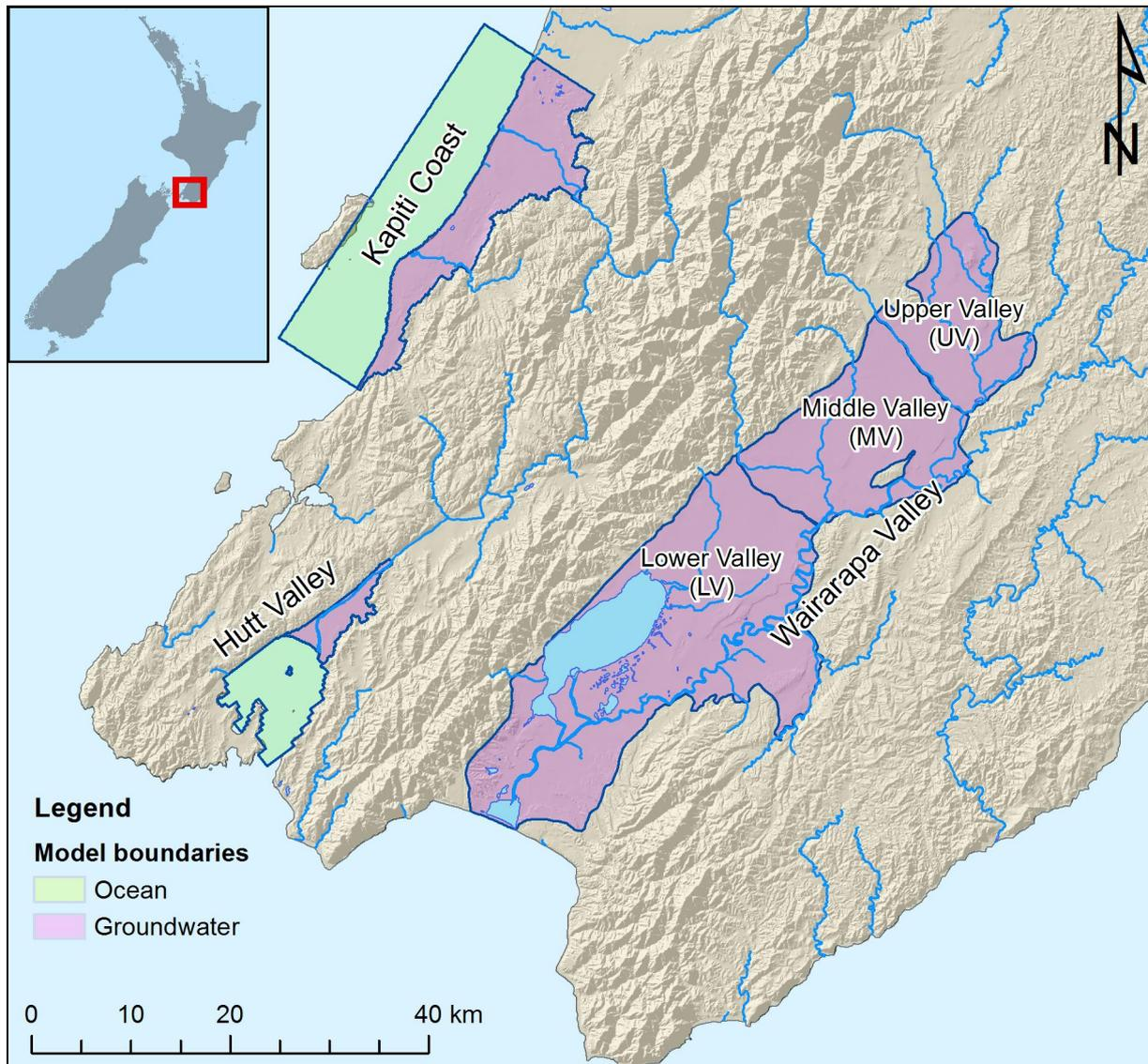
Figure 3: Geographical setting and model domains. Ocean boundaries are simulated with constant heads on the uppermost layer, and groundwater or inactive cells beneath. Outer inactive cells from each model are not shown.
