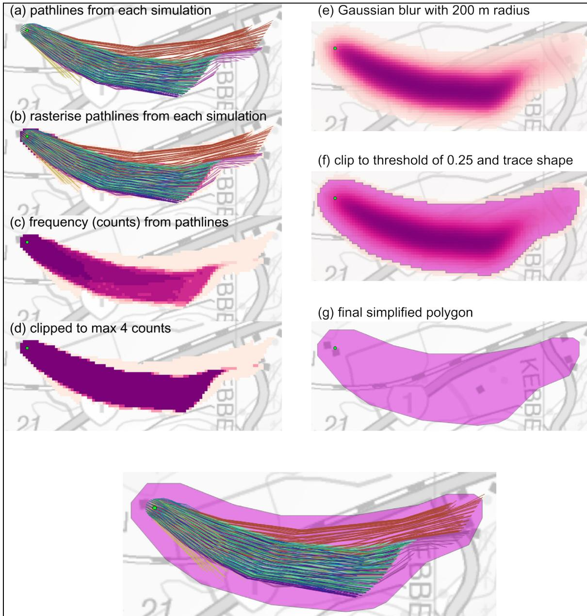
Figure 7: Processing for backwards pathlines to make a capture zone polygon, described in text. Subfigures (a) and (b) show different coloured lines that show pathlines to a pumped well from different sensitivity analysis simulations. Subfigures (c) to (f) show colour shading from light pink to dark purple, which represents a frequency or intensity of values of a raster. The purple polygons in subfigures (f) and (g) show the capture zone polygon.
