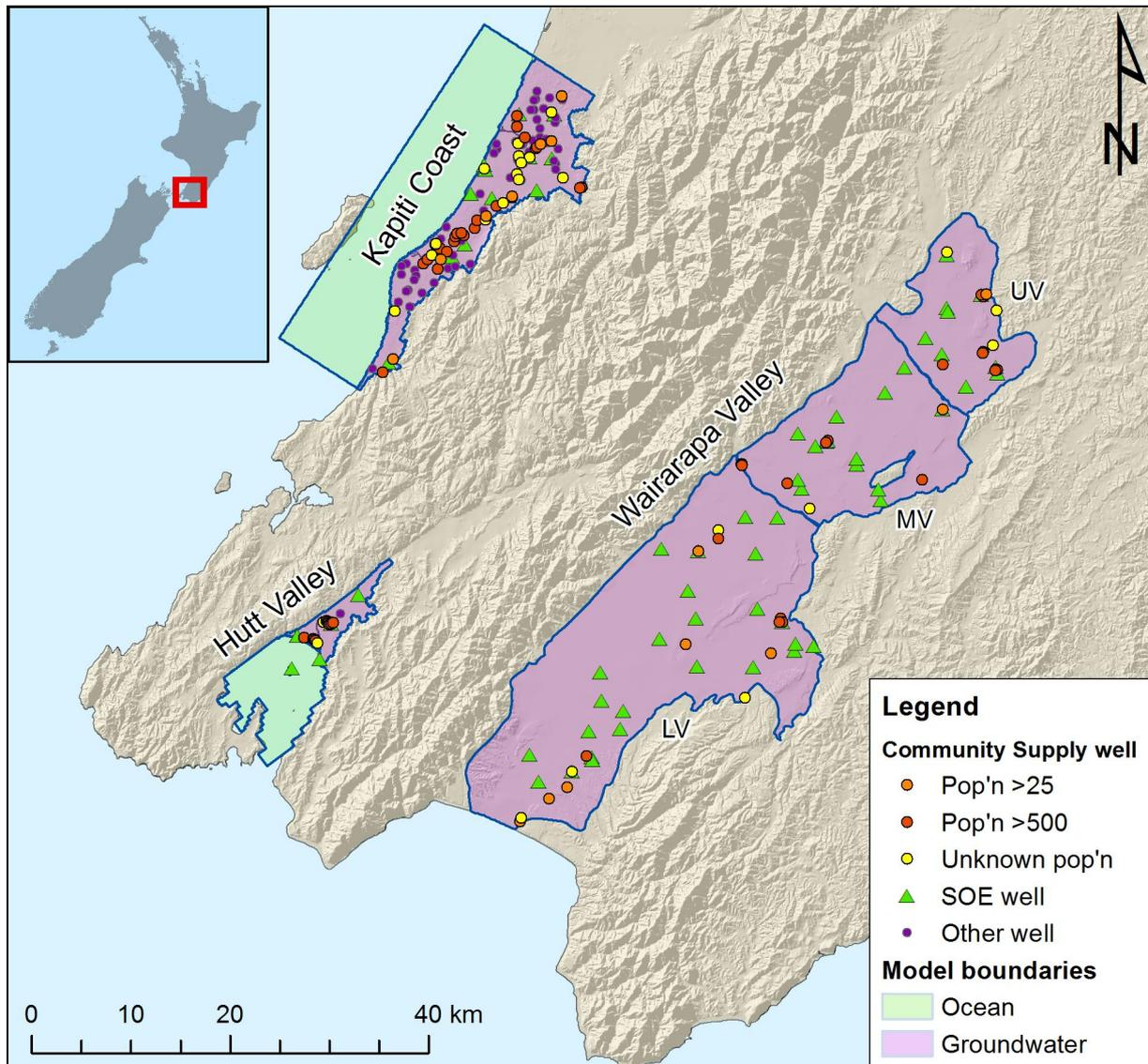
Figure 4: Well locations within the respective model domains: showing community supply wells based on population (pop'n) thresholds, State of the Environment (SOE) wells, and other wells that are not either SOE or community supply wells. Note that some SOE wells are also community supply wells, and have stacked symbols.
