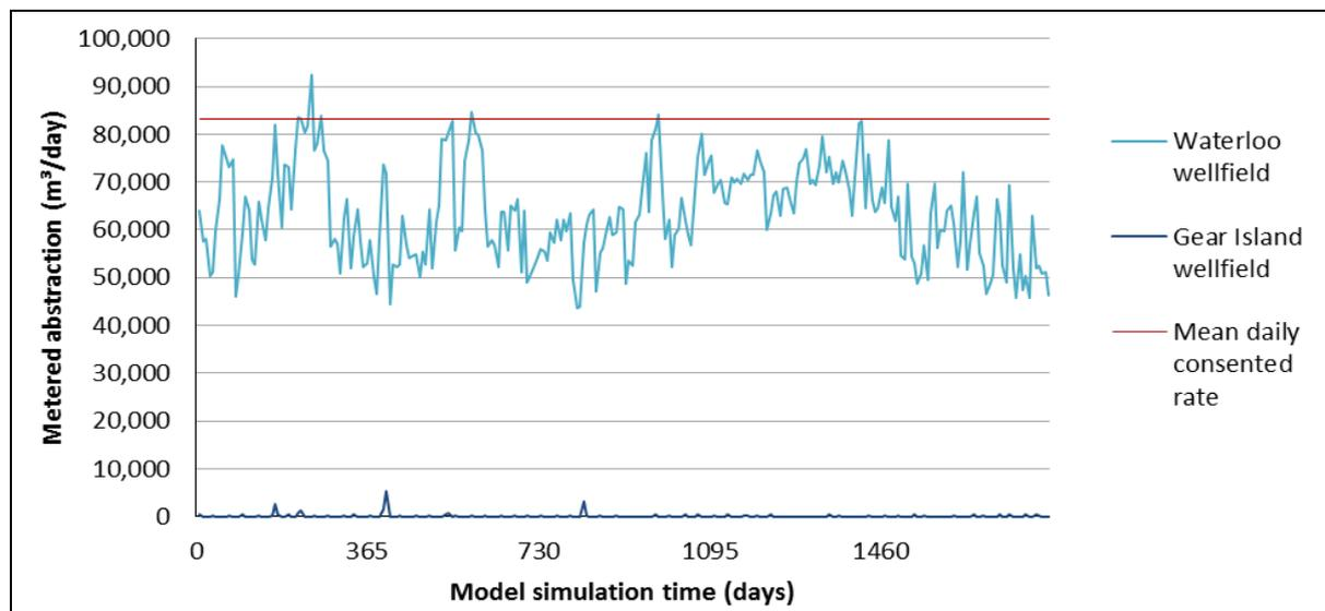
Figure 5: Metered abstraction of the Waterloo and Gear Island wellfield over the simulation period in comparison to the mean daily consented rate over a moving 12-month period (red line). The maximum consented limit (not shown) is 115,000 m³/d.
