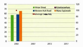
Figure 98: Noise adjacent to arterial routes (noise level 24hr  $\rm L_{eq'}$  dBa, one-week average). Source: GWRC survey, 2002
