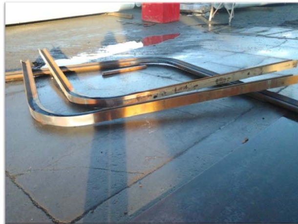
Rail irons successfully bent
