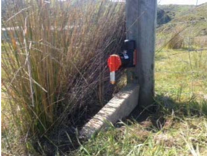
Image 5: Raised Goodnature A24 trap at Pencarrow so that dispatched hedgehogs roll away and clear the trap entrance.
