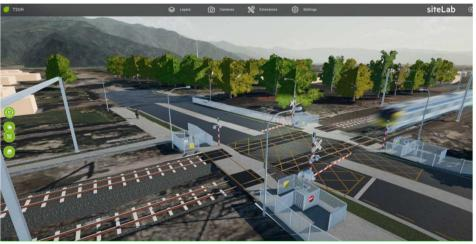
Image taken from Digital Engineering 3D model of Wallaceville level crossing
