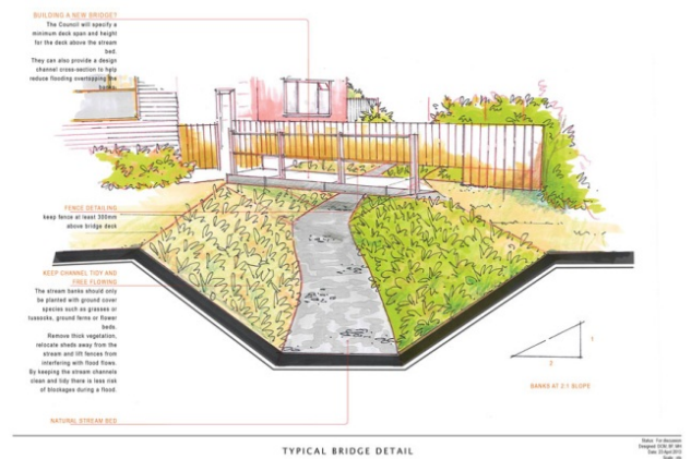
Figure18: Typical cross section of replacement bridge
