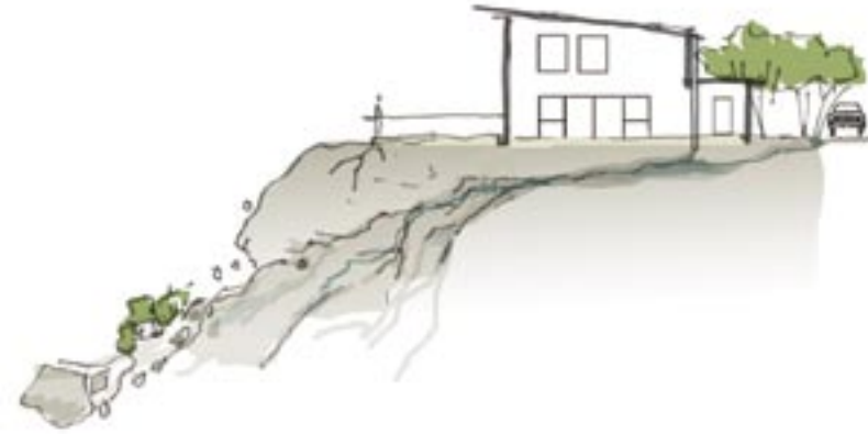
Uncontrolled stormwater runoff can lead to potential slips.
