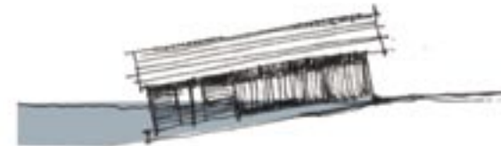
Wet areas can be susceptible to subsidence and uneven settlement when loads are imposed.
