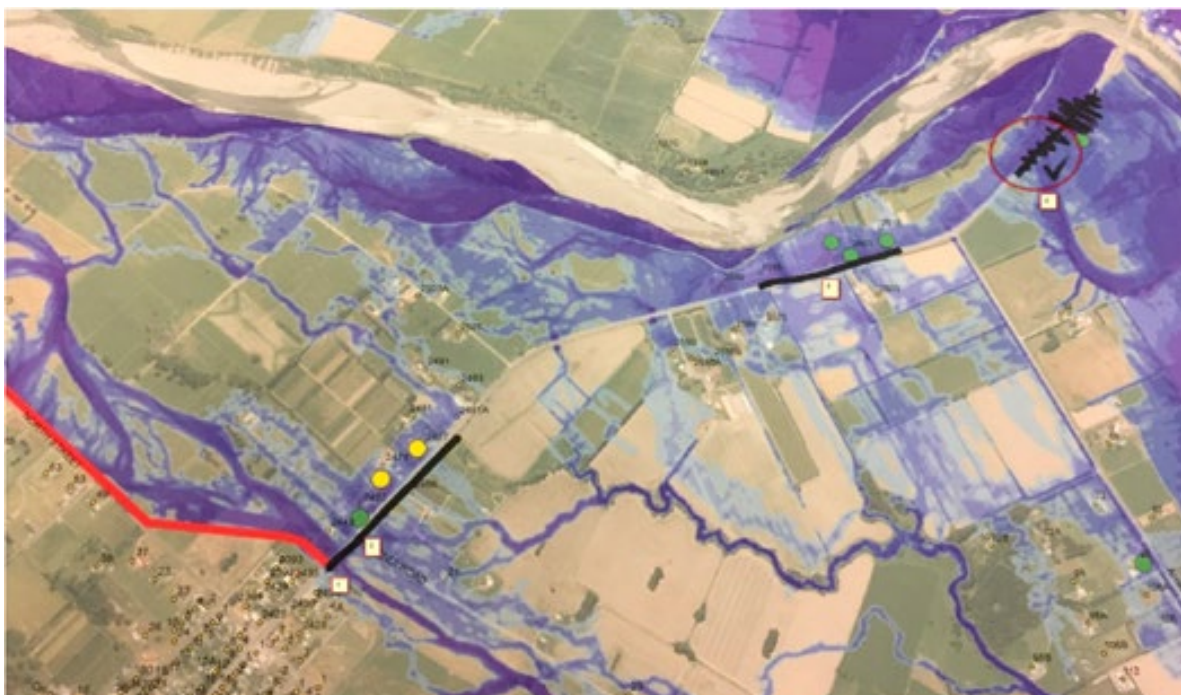
Figure 74: Flood Map – Detailed Study of need to raise crown of SH2 – landriversea Consulting.
